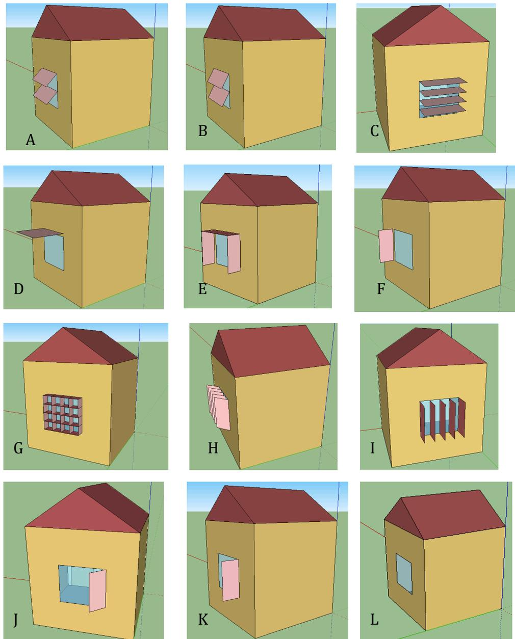
Figure 13 - Variations of Shading Devices analyzed
