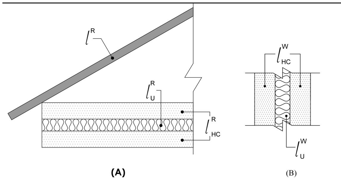
Figure 12 - Roof (A) and wall (B) virtual construction scheme. Source: Favretto, 2015.
