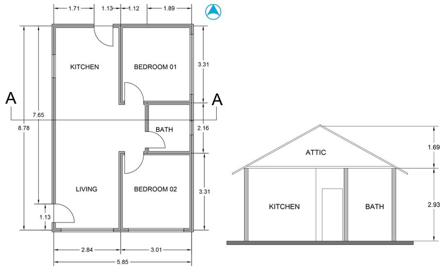
Figure 5 - Floor plan and Section A-A of base model in meters
