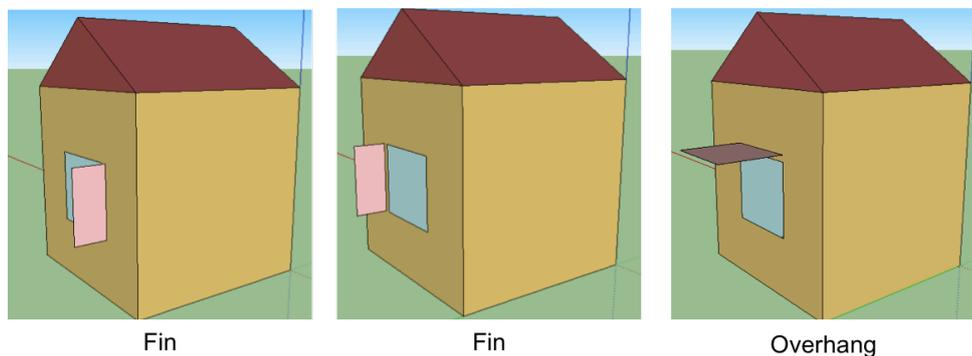
Figure 10 – Possible Shading Devices
