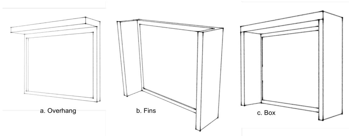
Figure 24 - Shading Devices Combinations considered in the tests
