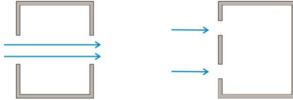
Figure 5: Cross-ventilation and single-sided ventilation examples.
